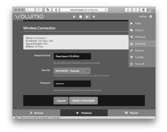
Enter the **exact** name (SSID) and WPA/WPA-2 Personal password of your wireless network and save these changes. The status information should confirm that you are successfully connected to your wireless network.
